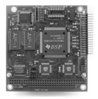
embedded DSP computer with the Model C32-104 performing functions normally done by the 80386 (or higher) CPU board. These functions include the controlling of PC/104 disk controller, RS-232 serial port, and analog I/O boards.
